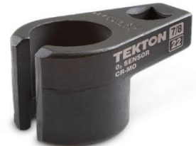
#889-1 OFFSET OXYGEN SENSOR SOCKET 3/8" DRIVE X 7/8" MADE FROM CHROME MOLYBDENUM PREVENTS DAMAGE TO WIRES
