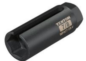
#889 OXYGEN SENSOR SOCKET 3/8" DRIVE COMMON 6 POINT, 7/8" (22mm) SIDE CUTOUT PREVENTS DAMAGE
